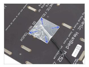
Maintain the thermistor position and cover it with aluminum tape.
