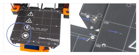
• Carefully inspect the surface of the heatbed. If you find any major scratches (up to the copper layer) consider replacing it with a new piece.
