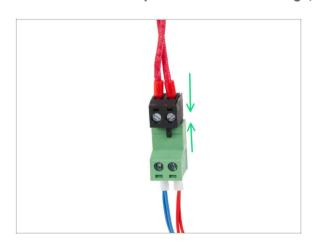
Connect the hotend heater cable to the green connector on the xBuddy cable adapter.
