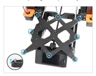
Install eight M3x6r screws in the outer holes on the Y-carriage. Do not tighten them completely. A few turns are enough for now.
