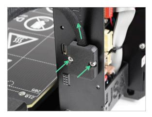
Attach the heatbed-cable-holder to the xBuddy box. The cable bundle must be pointing up. Secure it by tightening both M3x6 screws firmly.
