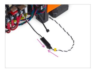
Plug the power panic guiding from the PSU into the power panic extended cable.
