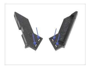
Insert two M3nS nuts into the xLCD-support-left and xLCDsupport-right.
