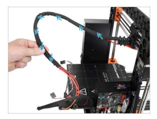
Twist the entire length of the textile sleeve. Twist the sleeve, not the cables!
