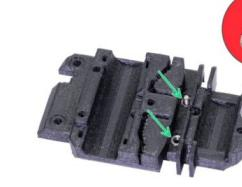
**⚠️** For the following nut insertion **USE A SCREW. THAT'S AN ORDER!!** Seriously, use a screw to pull the nuts in, both have to be properly seated in the X-carriage.
