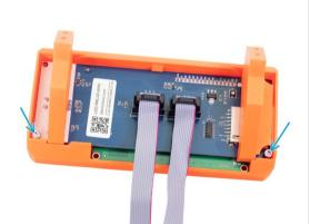
Using the 2.5mm Allen key and two M3x10 screws, secure the LCD controller in place.
