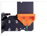
WARNING: Printed parts aren't the same! There is a left and right oriented piece. See the markings on the parts. Also note the correct orientation of the frame, the "PRUSA" logo and the safety sticker must be facing towards you.
