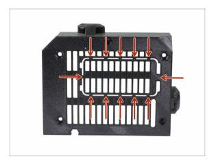
Einsy-base has a maintenance opening for the RPi Zero W or RPi Zero 2 W. If you intend to use this mini computer, you can carefully cut the piece of the plastic now. More details here:
