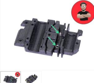
⚠ For the following nut insertion **USE A SCREW. THAT'S AN ORDER!!!** Seriously, use a screw to pull the nuts in, both have to be properly seated in the X-carriage.
