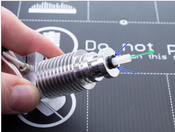
**⚠ THIS STEP IS OBLIGATORY!** The MK3S+ is using a shorter PTFE tube compared to the MK3S, let's replace it now!
