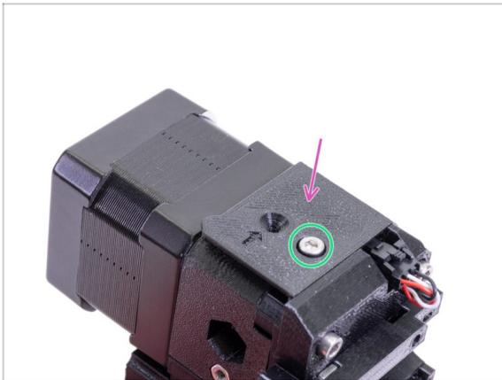
◆ Place the FS-cover on the extruder and align it according to the picture.
