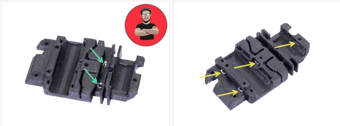
**⚠** For the following nut insertion **USE A SCREW. THAT'S AN ORDER!!!** Seriously use a screw to pull the nuts in. Both have to be properly seated in the X-carriage.
