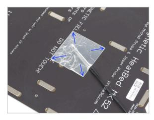
Maintain the thermistor position and cover it with aluminum tape.
