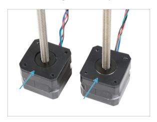
Place both rubber pads onto the motor surface. Make sure the holes in the pads are aligned with the holes in the motors.
