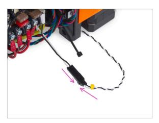
Plug the power panic guiding from the PSU into the power panic extended cable.
