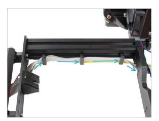
Guide both cables through the cable clips on the inside of the frame.
