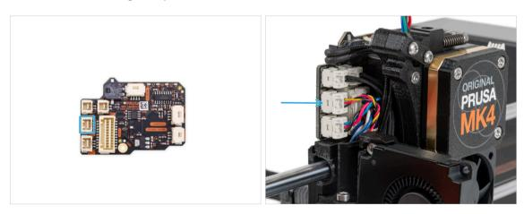
• Connect the print fan cable to the middle slot on the left side of the Loveboard.
