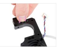
Insert the Prusa ball holder assembly into the heatsink. Make sure the steel ball part is closer to the side of the heatsink.
