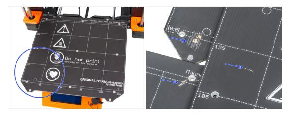
Carefully inspect the surface of the heatbed. If you find any major scratches (up to the copper layer) consider replacing it with a new piece.
