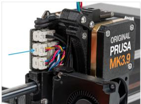
• Connect the print fan cable to the **middle slot** on the left side of the Loveboard.
