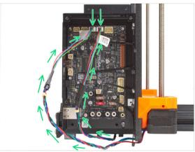
Connect the cables to the third and fourth slots on top of the xBuddy Board.
