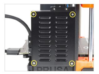
Align the xBuddy box cover with the xBuddy box and secure it with four M3x6 screws.
