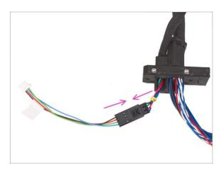
Plug the X motor cable guiding from the Ext-cable-holder to the motor cable adapter.
