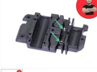
⚠️ For the following nut insertion **USE A SCREW THAT'S AN ODD SIZE!** (Normally, use a screw to pull the nuts in, both have to be properly seated in the X-carriage.)
