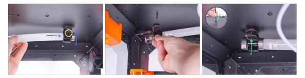
Insert the metal end of the tube into the P-clamp.
