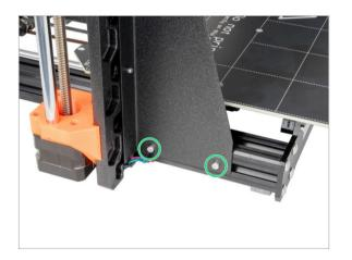
Fully tighten the screws on the printer frame support.
