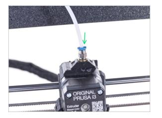
Insert the free end of the PTFE tube to the Fitting QSM-M5 on the extruder. Insert it all the way down.
