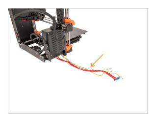
Place the printer back on its feet. Place the PSU cables next to the printer. We'll come back to them later.
