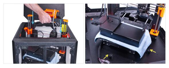
• Grasp the printer by its frame and carefully insert it into the enclosure at a slight diagonal angle to **avoid scratching the printer and enclosure.**
