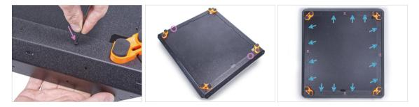
Secure the bottom panel near front and rear corner by two M3x4 screws.
