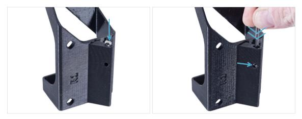
Insert the M3nS nut into the External-PSU-bracket-XP. Using the Allen key, push the nut all the way into the printed part and align the nut with the hole in the part.
