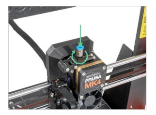
Insert and screw the Fitting QSM-M5 directly into the threaded filament hole in the extruder.
