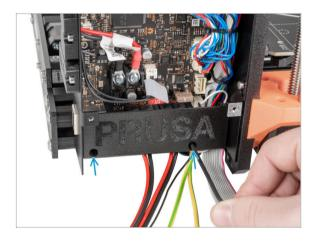
Using a 2,5 mm Allen key, tighten two M3x10 screws.
