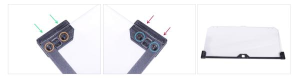
Do not overtighten the screws in the door panel! The panel could crack.
