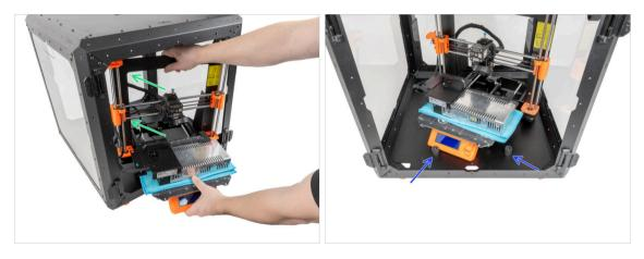
To get the printer into the enclosure, insert its left side first.
