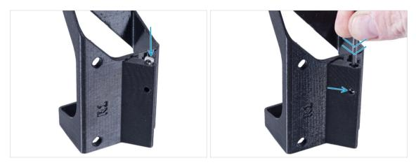
Insert the M3nS nut into the External-PSU-bracket-XP. Using the Allen key, push the nut all the way into the printed part and align the nut with the hole in the part.
