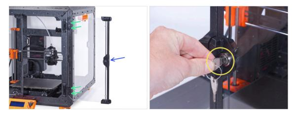
Do not overtighten the screws in the door panel! The panel could crack.
