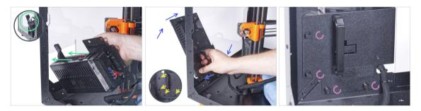
• From inside the enclosure, grasp the PSU by its handle.
