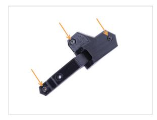
Insert three M3n nuts into each hinge assembly.
