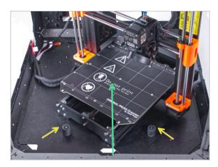
• To get the printer into the enclosure, insert its left side first.
