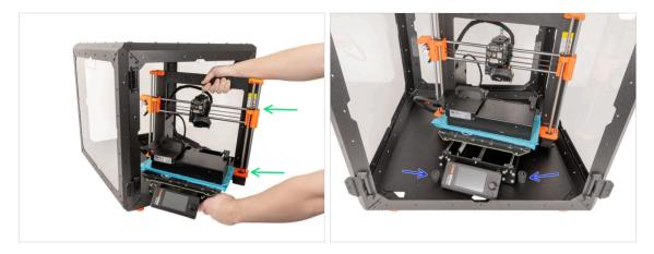
• To get the printer into the enclosure, insert its left side first.
