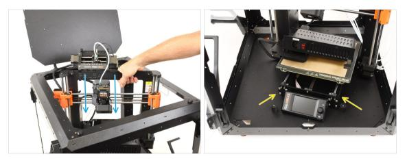
Grasp the printer by its frame and carefully insert it into the enclosure at a slight diagonal angle to prevent scratching both the printer and the enclosure.
