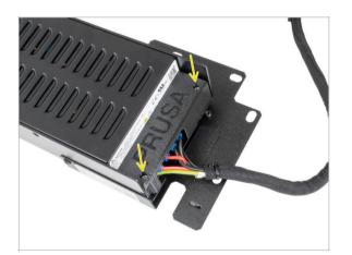
Mount the PSU cover back on the PSU using two M3x10 screws.
