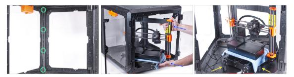
In the same way, guide the filtration cable alongside the rear left support profile and secure it with four zip ties.
