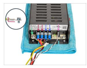
Place the single end of the PE cable (not the forked end) in the same position as it was removed. Secure the cable by re-using the screw and washer.
