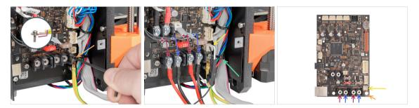
• Using a 2,5 mm Allen key, secure the PE cable with the M3x6 screw with a washer.
