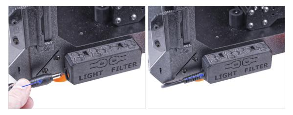
• Connect the external PSU cable to the basic board from the left side.
