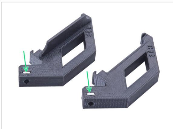
Insert all the way the M3x10 nut into each LCD-support.
