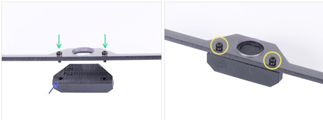
**⚠ Do not overtighten the screws in the door panel! The panel could crack.**
