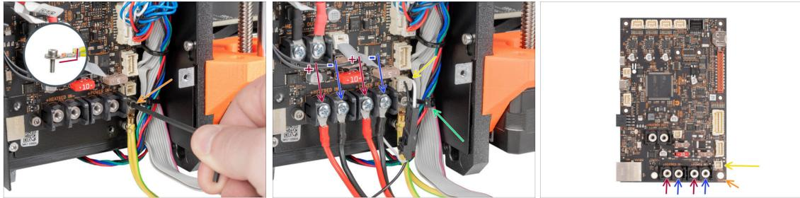
Using a 2,5 mm Allen key, secure the PE cable with the M3x6 screw with a washer.
