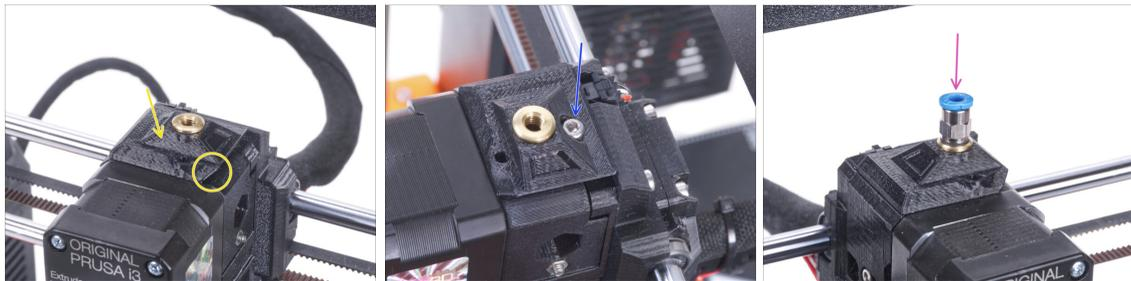
◆ Attach the new FS-cover on the extruder. See the correct orientation. The beveled side must be on the right (above the extruder-idler).
