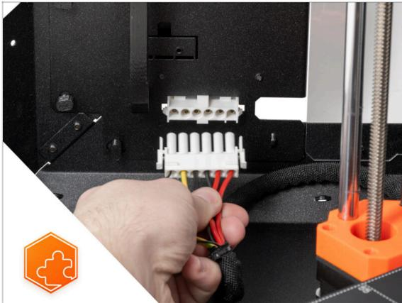
● This guide will take you through the installation of the **Quick release PSU cable** on the **Original Prusa Enclosure**.
