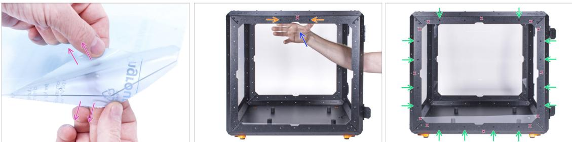
● There are protective foils on both sides of the panel. Peel off both foils.
