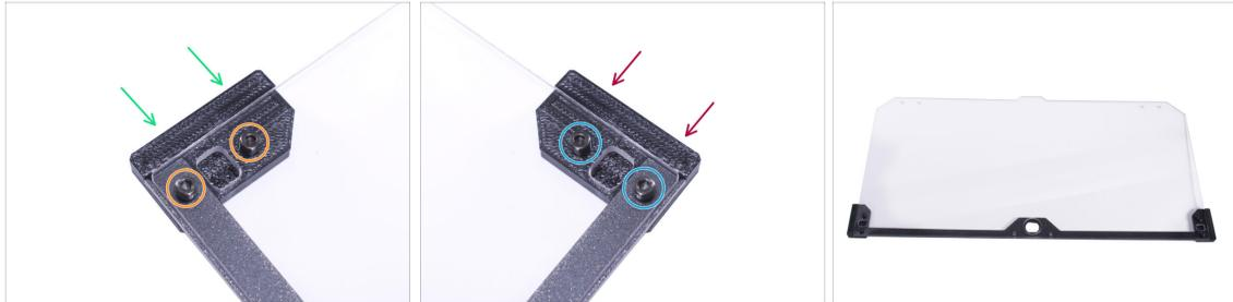
⚠ **Do not overtighten the screws in the door panel! The panel could crack.**
