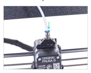
Insert the free end of the PTFE tube to the Fitting QSM-M5 on the extruder. Insert it all the way down.
