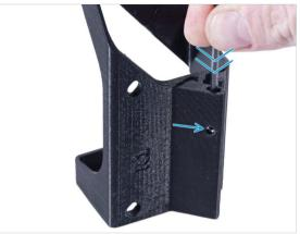
Insert the M3nS nut into the External-PSU-bracket-XP. Using the Allen key, push
