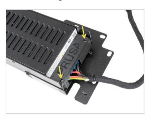
Mount the PSU cover back on the PSU using two M3x10 screws.
