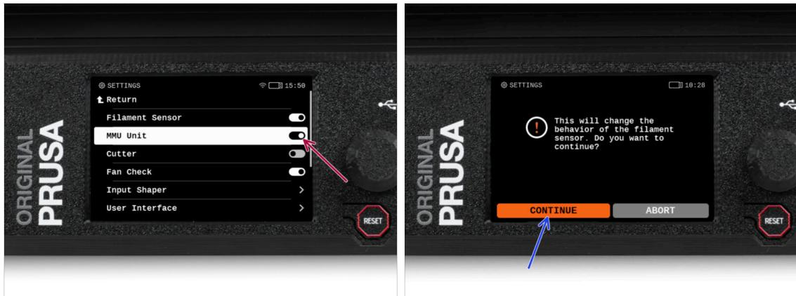
**⚠ After finishing the firmware update, make sure there are no filaments loaded neither in the extruder, or in the MMU unit.**
