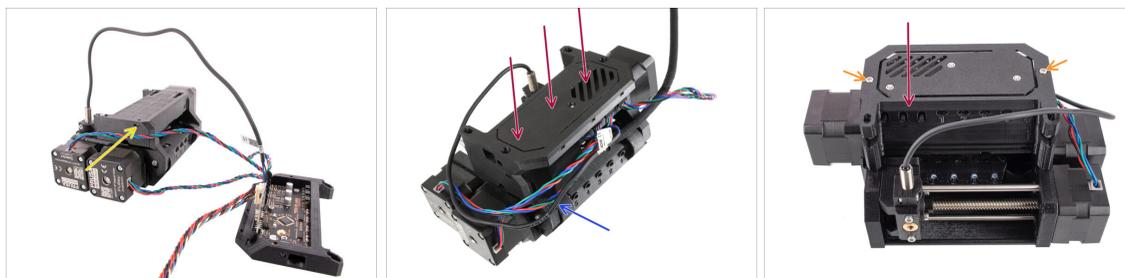
● Insert the **M3nS nut** into the marked opening and press it all the way in.
