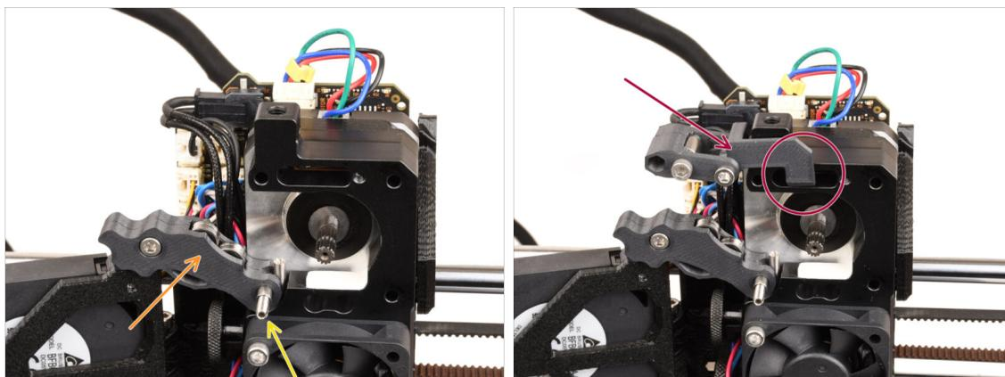
◆ Add the **Idler assembly** onto the extruder.
