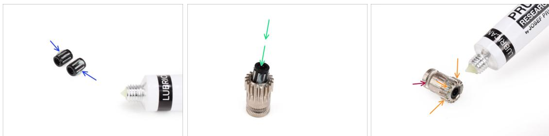
Add a **tiny bit of lubricant** into the needles in both of the bearings. Wipe off the excess grease to prevent spreading it all over the place.
