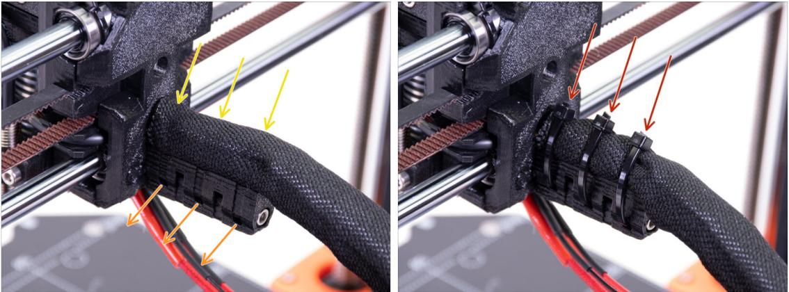
● Gently twist the sleeve to tighten it up around the cables. Slide the sleeve towards the extruder.
