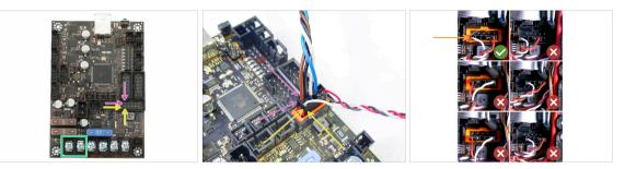
Note the marked position. The MMU Signal cable connector should go here. (upper row of the pins, brown wire in the plug must be facing left)
