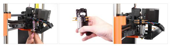
Re-insert the hotend back into the extruder. Ensure its orientation is the same as seen in the picture.
