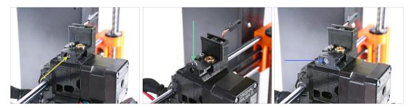
Insert the M3x30 screw into the marked opening on the side of the Chimney Base.
