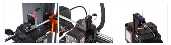
Attach the IR filament sensor onto the top of the chimney.
