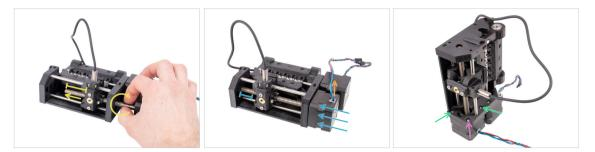
Rotate the threaded rod while pushing it towards the selector to engage it into the trapeze nut.
