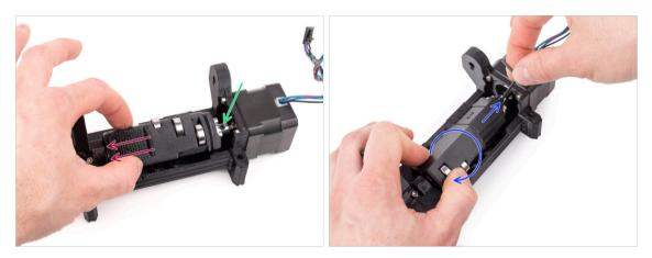
• Pull the idler to the side all the way away from the motor. There should be just a very small gap on the left side.
