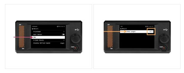
The MMU-to-Extruder PTFE tube length needs to be set in the firmware.
