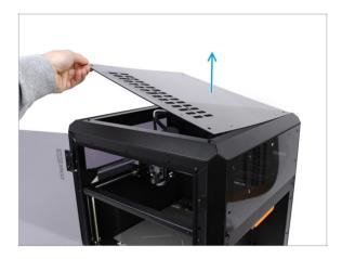
Before installing the MMU unit, remove the printer's top cover if it hasn't been removed already.
