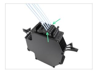
Insert the PTFE tubes into the row of collets on the right of the cartridges. Push them all the way in.
