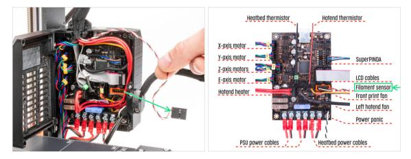
Carefully unplug the IR filament sensor cable and make sure it is free inside the electronics box.
