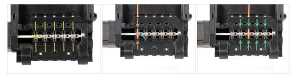
WARNING: this step is crucial in order for the MMU unit to work properly! Please check your pulley alignment multiple times!!!
