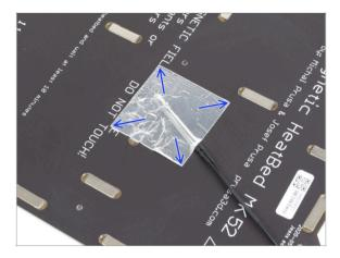
Smooth out the aluminum tape around the thermistor using your fingers only, to ensure it is fully adhered.
