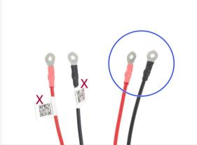
• Follow the polarity markings on the heatbed:
