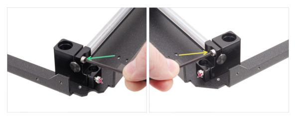
Focus on the front left holder (now on the right) and secure the rod by tightening the screw in the holder.
