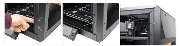
From the inside of the printer, insert the magnet holder assembly into the corresponding bottom opening in the right-side metal profile.
