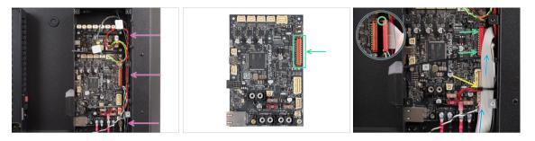
Arrange the cables as shown - route all cables along the right side of the xBuddy box.
