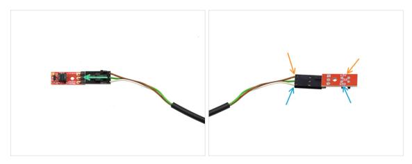
Plug the cable into the IR filament sensor.
