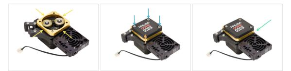
• Apply more grease between the gears if your gearbox lacks lubrication.
