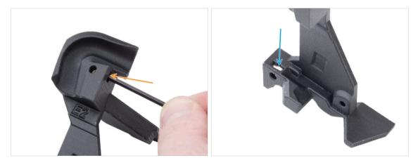
Locate the U-shaped cable channel on the Loveboard-mount and insert an M3nS nut into the nearby hole.
