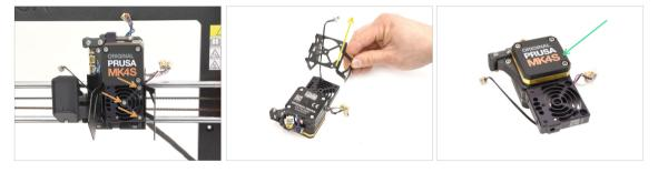
• Remove the three screws holding the Nextruder to the X-carriage.
