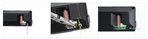
• Let's move on to the fourth screw opening—this is where we will attach the grounding faston connector.
