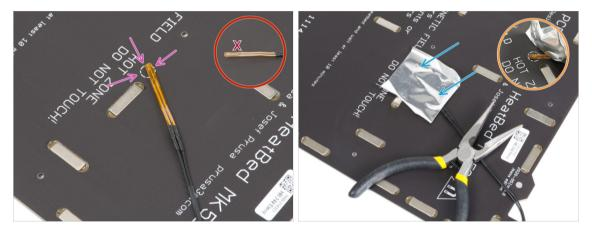
Place the thermistor onto the heatbed, ensuring the tip is positioned inside the circle.
