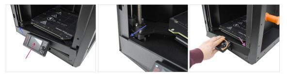
Gently lift the xLCD assembly into the upward position.
