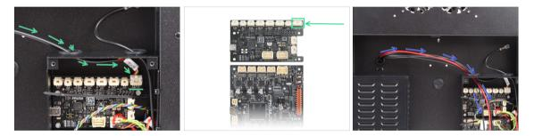
Route the RGB LED strip cable through the left hole in the xBuddy box and connect it to the first slot on the xBuddy board labeled 'RGBW LED.'
