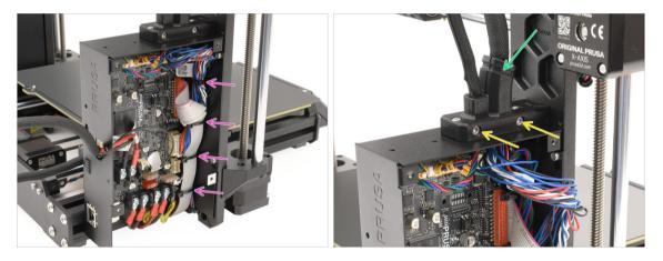
Remove all the zip-ties securing the cable bundle inside the xBuddy box.
