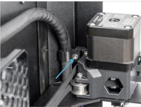
• Fix the main-cable-clip with the cable to the hole using the M3x10 screw.
