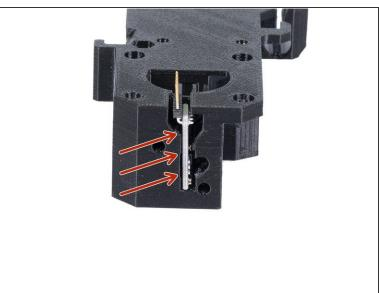
Carefully insert the filament sensor in the slot, do not use force or you might damage the PCB!
