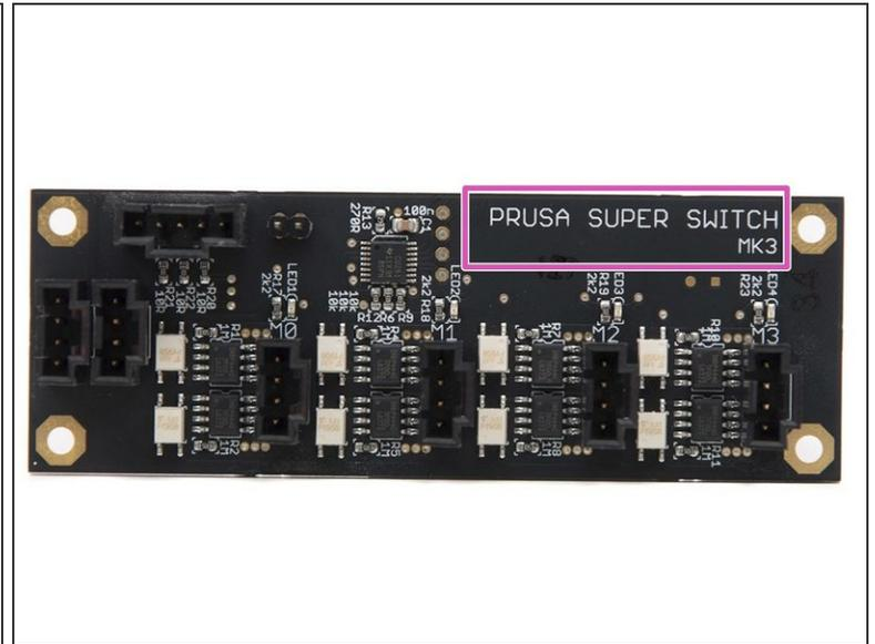
**⚠ Starting 3rd of August 2017 the Multi Material upgrade is shipped with new a electronics board** for the Extruders. Main difference is in the size and layout of the connectors. Functionality is the same.
