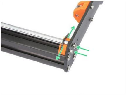
**⚠ IMPORTANT:** proper alignment of the smooth rods is crucial to reduce noise and overall friction.
