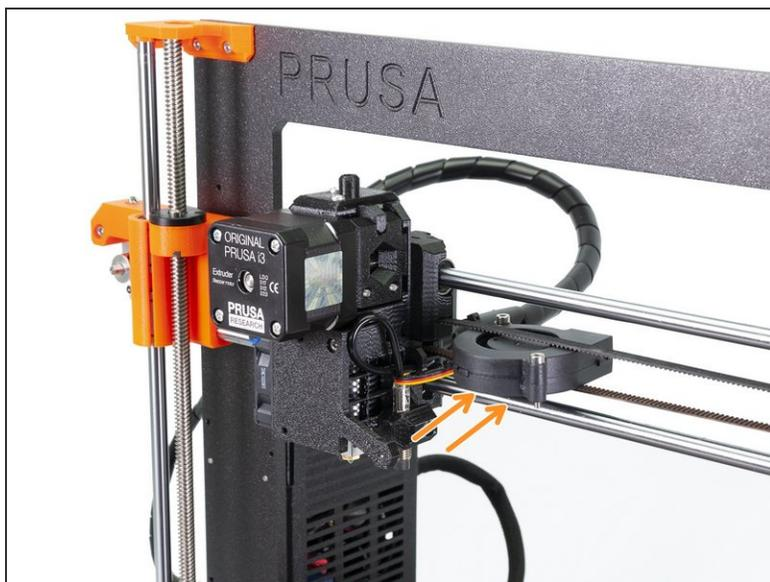
**⚠** Ensure the **filament is not loaded** in the hotend. **Remove it** before proceeding further.
