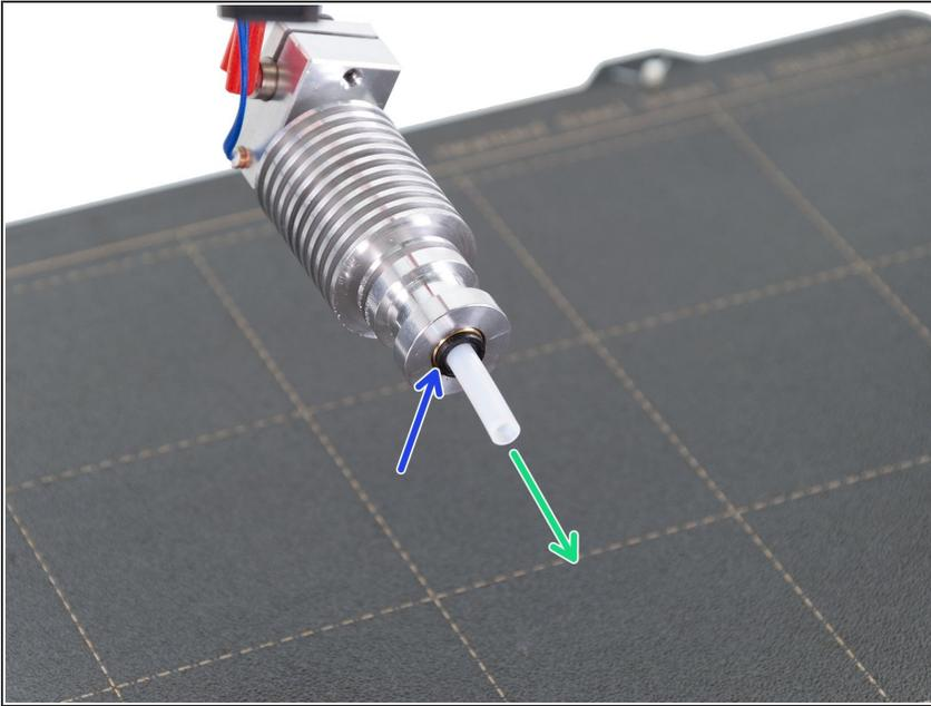
**⚠ This step is optional**, however if you have a spare PTFE tube it might be a good time to check your current tube for any defects and if needed replace it.
