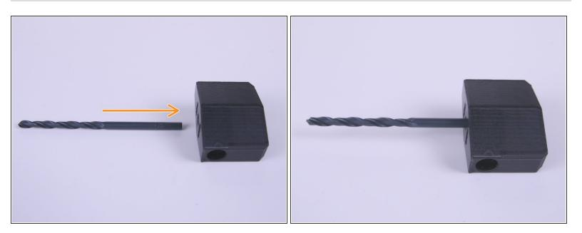
Insert the 3 mm drill bit all the way into the P-drill printed part.
