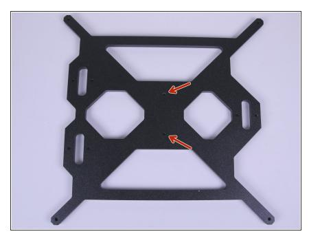
Highlighted holes are going to be drilled in next steps.
