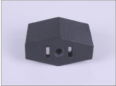
• Insert M3nS square nuts into the nut traps in the P-drill printed part.
