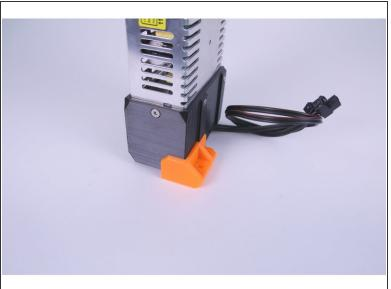
Press the PSU-reinforcement with glue on your power supply and wait until the glue dries.
